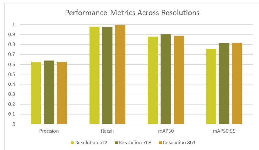
Figure 7. Comparison of achieved metrics (Precision, Recall, mAP@50, mAP@50–95) across three training runs using input resolutions of 512, 768, and 864.
