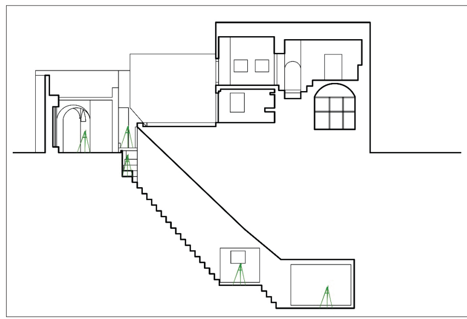
Figure 6. Schematic Position of Measurement Equipment at Various Depths of Shavadans.
